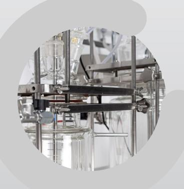
REC reactor units are made either of glass, stainless steel (optional steel enamel also available) or C22 nickel alloy. Surface is treated to pharma-quality with electropolishing. We make them as mobile or fixed units. They can be fully or partially automated with modern control and regulation systems connected to the existing central control systems. The reactors are adapted to the needs of the customer according to the equired process parameters.
